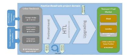
The image above shows the variety of urban biogenic feedstock that can feed the HTL process and the end products that can be obtained. The potential total feedstock amounts to about **107 M dry ton per year only in the EU**. Specifically, sewage sludge equal to 13 Mton, construction wood waste 6 Mton, and food waste to 88 Mton. In the EU 27, sewage sludge is produced at the **rate of 24.3 kg/pe/year**, where pe is the population equivalent served by WWTP.
