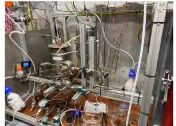
Reactor Operation temp 620 °C and 220 bar
