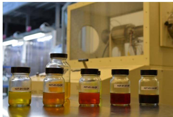
Figure 1: Hydroprocessing of HTL biocrude from Spirulina algae in a two-stage reactor with graded catalyst bed operating at different conditions (i.e., WHSV, T and P).
