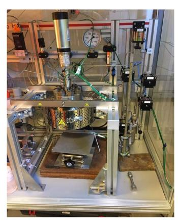
Catalyst testing in high pressure batch reactor and product analysis by NMR
